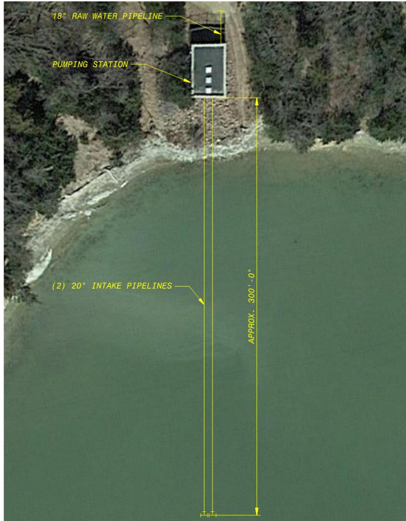
INTAKE/PUMPING STATION NO. 1 1" = 500'-0"
