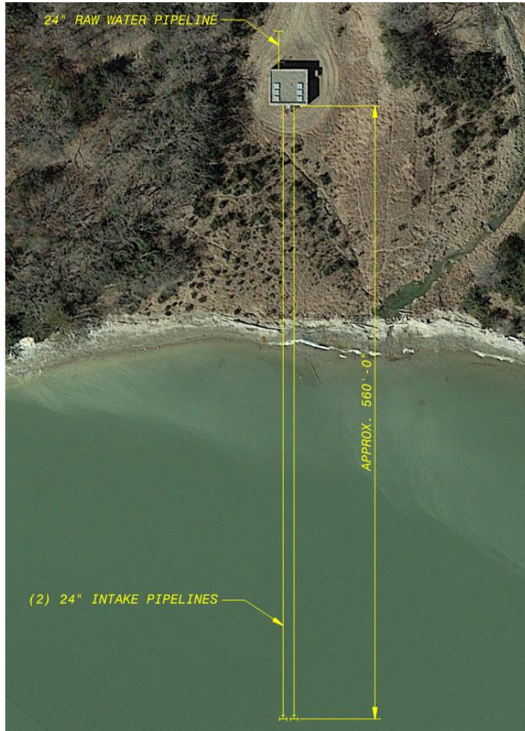
INTAKE/PUMPING STATION NO. 2 1" = 1000'-0"
